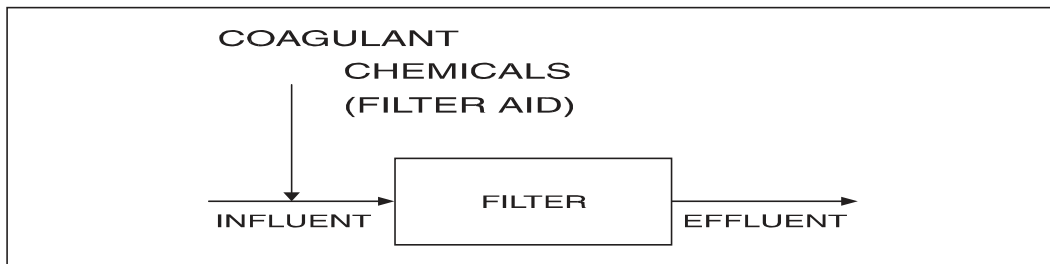
Fig. 6.4 - IN LINE FILTRATION
